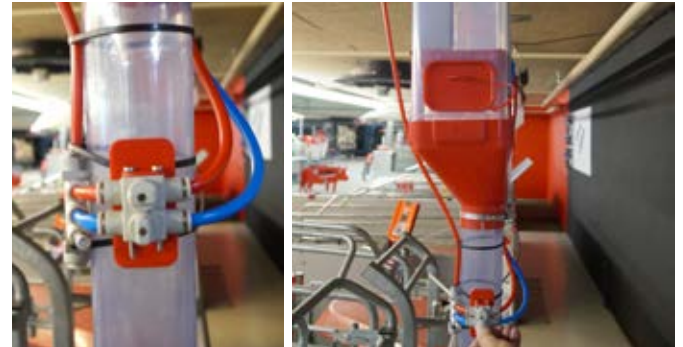
COLOR FEED SINGLE: Fasefodringsventil i farestald
